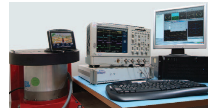
Typical test system using a GSS6560 with SimAUTO driving a rate table & producing wheel ticks
