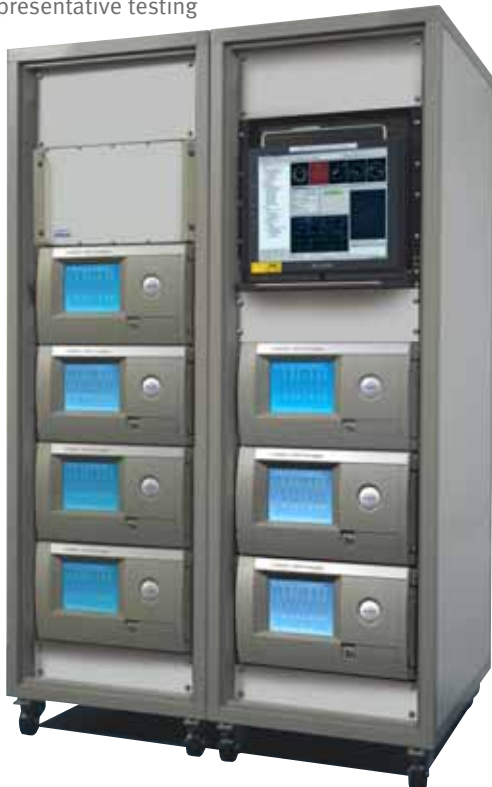
Spirent GSS8000 7 element CRPA test system
