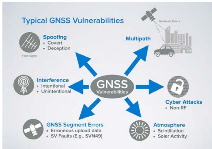
The many sources of GNSS interference
