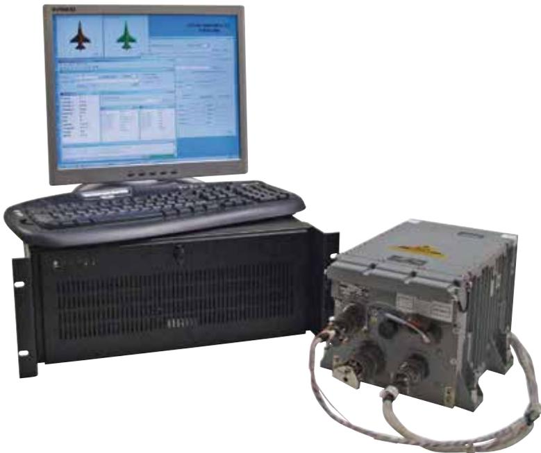
**SimINERTIAL\*:** Operational performance of an Integrated GPS/ Inertial (IGI) system can be established in the laboratory using real-time emulation of the inertial sensor outputs along with a GSS8000 constellation simulator. All signals are coherently generated to exactly match the simulated vehicle trajectory. Typical inertial sensor performance can be represented by a sensor error model driven by the simulated motion, with appropriate coefficients entered by the user.
